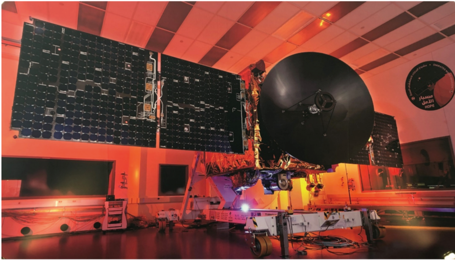
Fig. 13 EMM Hope Probe undergoing solar array testing
