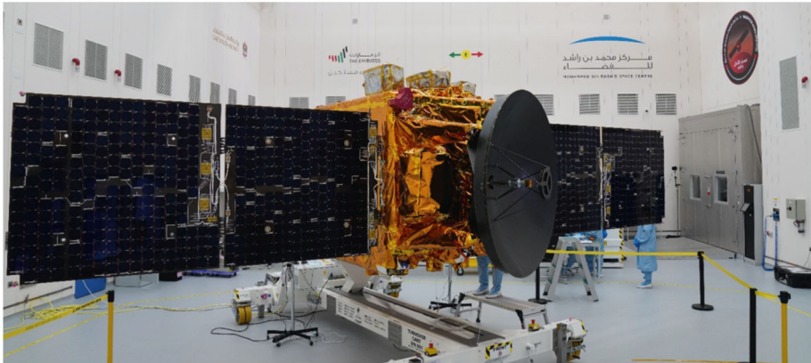
Fig. 21 EMM observatory solar array deployment testing
